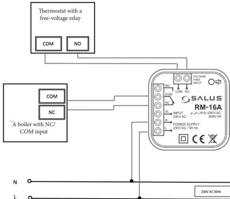
3. Connection of the receiver transmitting power higher than it is allowed by the relay in a regulator. The maximum electricity consumption of the receiver cannot exceed 16A
