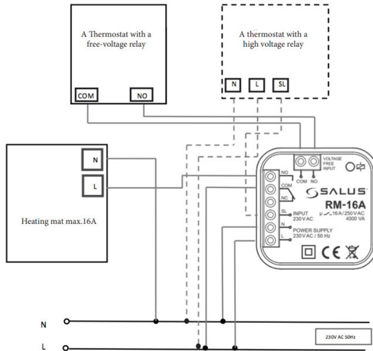
4. Connection of the devices other than electro thermal actuators with the wiring centre (KL06-M / KL08NSB / KL08RF / KL10 / KL10RF) e.g. if you want to connect a pump or an electric heating mat instead of a electro thermal actuator.
