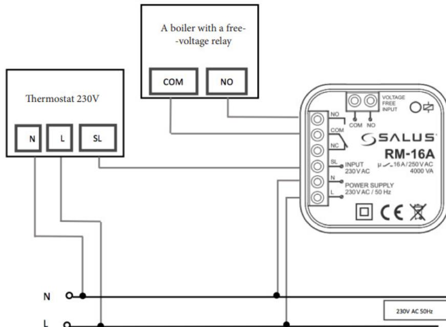
2. Connection of the SALUS temperature regulator with NO/COM relay (e.g. 091FL) with a boiler control which requires NC/COM output ( NC/COM output is normally required in solid fuel boilers controls).
