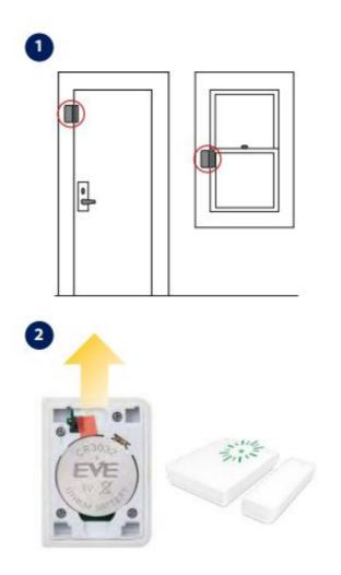
After removing the plastic battery tab, the LED will flash green intermittently.
