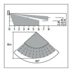
The Motion Sensor should be placed in a corner of the room with a view of each entry point. For accurate motion detection, there should be no obstacles in front of the product's lens. The mounting height must be between 1.9 m and 2.3 m.
