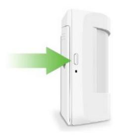
Press the reset button for 3 seconds then release the pin to reset the sensor. After the reset, the sensor will be found by the App or the gateway when they search for the device.
