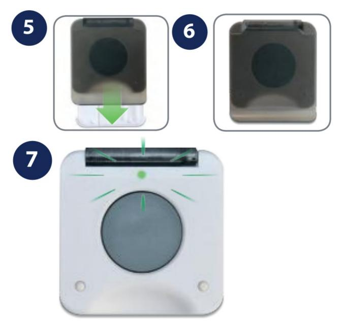
During initialisation, the LED lights up for 2 seconds, then will flash until the network is found (max 20 times). When joined the LED will go off.
