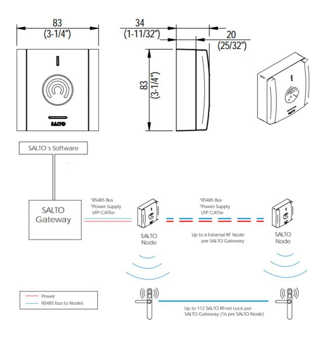
• The BLUEnet Node and RFnet Node are part of SALTO wireless system. They work as a bridge, with the SALTO Gateway, between SALTO's access control software and wireless locks.
