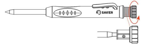
3. step3: Install the pencil lead, press pencil lead release button to the bottom, insert the pencil lead from the bottom.
