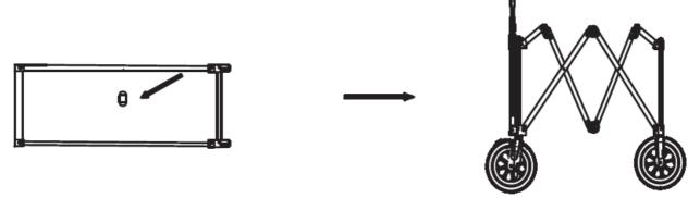
4. When not in use, press the "press" button on the pull rod to shorten the pull rod; Pull out the pull rod directly during use. The pull rod can hover and be stressed at any position within 90 degrees, so that it can be used by people of different heights.
