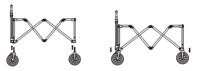
Brake instructions: firmly press "lock" to lock the wheel, and gently press "unlock" to unlock it. (Note: do not use the brake on the ground with a gradient greater than 5 degrees.)
