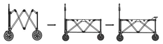
3. Folding and storage: after taking out the folded bottom plate, gently lift the bottom center pull ring, and the frame will automatically gather.
