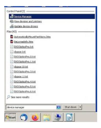
3. In Device Manager, locate the "Ports (COM & LPT)" entry and click it to display the active driver that is in use. For this CNC control boards, it should be "CH340", but it may display different COM port numbers. Make a note of the COM port number as it will be needed later.
