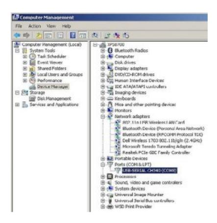
4. Double-click the highlighted driver line to expand it. When expanded, it will display multiple tabs, click the Port Settings tab and set it to transfer at 115200 bits per second.
