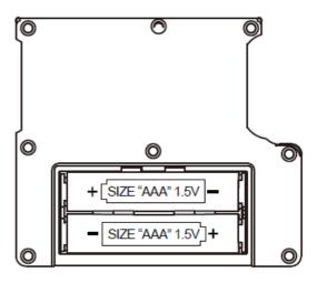
1. Open the battery cover on the battery compartment and insert 2pcs AAA batteries (not included, need to purchase additionally). Remember to check for the correct polarity(+/-).
