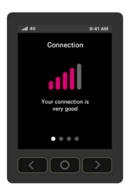
Like your phone, the gateway displays up to five bars on its Connection screen, indicating signal strength.
