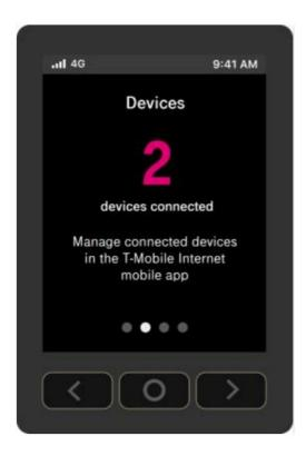
The Devices screen indicates how many devices are currently connected to the gateway. This is true for both wireless and wired devices.
