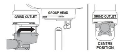
To start the auto grind, dose & tamp function, rotate the portafilter to the right then gently guide back to the centre position. Grinding will commence.
