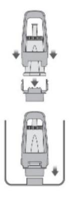
• Fill the water tank with cold water before sliding back into position at the back of the machine and locking into place.
