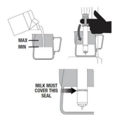
To start, press down and release steam lever. Milk texturing will stop automatically when the selected milk temperature is reached. Lift steam wand to remove milk jug. Wipe the wand and tip with a damp cloth. Lower steam wand to the down position and the wand will automatically purge.
