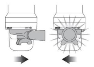
When the auto grind, dose & tamp function is complete, rotate the portafilter handle to the INSERT position and lower to remove.
