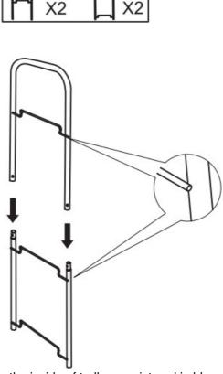
Ensure that basket securing rails face the inside of trolley as pictured in blowup diagrams of steps1, 2 & 3
