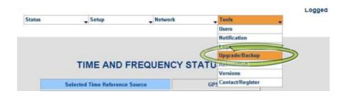
5. Ensure the Software/License Upgrade tab is orange (Orange indicates the tab is selected). Either click in the blank text box located next to Upload File, or select Browse to be able to select the update file (see illustration below).
