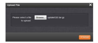
Note: When uploading files remotely via long distances, or when uploading multiple files via several browser windows simultaneously, the upload process may fail to complete. In this case, cancel the upload by clicking X, and go back to Step 2.
