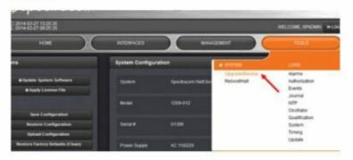
Click on the button Update System Software in the top-left corner. The Upgrade System Software window will open (see illustration below):
