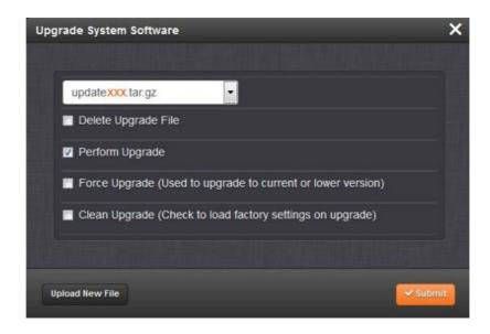
Force Upgrade — When checked, will force the software to install all update packages, even if it is already at the current revision, (for example, it is desired to install version 5.9.8, even though version 5.9.8 is already installed). The software will reinstall over the previously installed packages.
