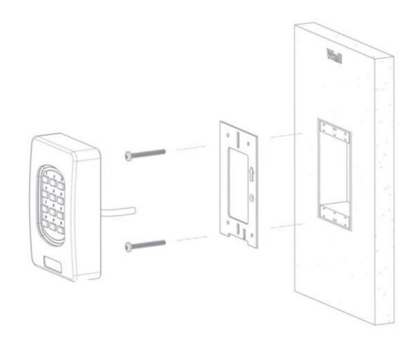
For a wall mounted installation, locate the electrical box which will be recessed into the wall. You will see a top and bottom metal flange with holes which is used to secure the back plate to the wall. Using the Phillips machine screws provided (#6- 32 x .375") screw the back plate against electrical box so that it's flush.
