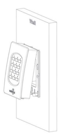
Once the back plate has been fitted and the wiring is complete, the top casing can be inserted onto the bottom casing like shown above.
