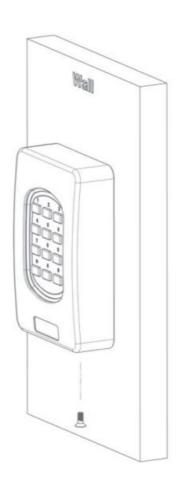
Complete the hardware installation by fixing the snake eye screws (security screws) to the top and bottom casing (#6-32X5/16" SS).
