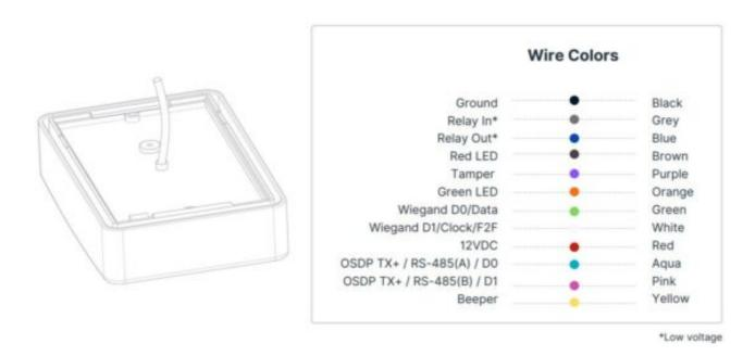
The next step is to connect the wires as per the wiring table above.
