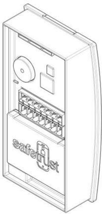
7. With the SABRE module connected, re-mount the reader onto the wall and reinsert the mounting screw.
