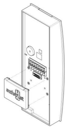
6. Once a connection is made between the Hiroshi connectors, the module will start to receive power and within 5 seconds will be operational.
