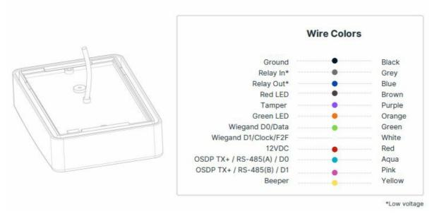
• The next step is to connect the wires as per the wiring table above.
