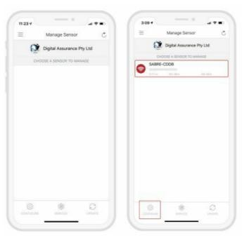
• With the Admin Installer tab open from the App, bring the phone in range of the IoT Sensor and once visible from the App, highlight and select "Configure".
