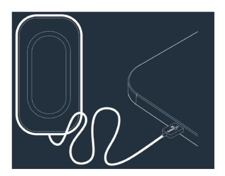
To install, simply uncoil the cord and plug the lot Sensor USB Reader/or Programmer into your laptop or desktop computer. Within 5 seconds, the loTSensor will complete its "power on cycle" and be operational and ready for configuration.
