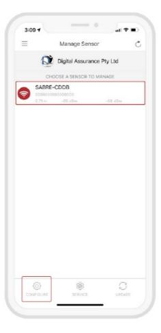
• With the Admin Installer tab open from the App, bring the phone in range of the IoT Sensor and once visible from the App, highlight and select "Configure."
