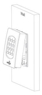
Once the back plate has been fitted and the wiring is complete, the top casing can be inserted onto the bottom casing like shown above.
