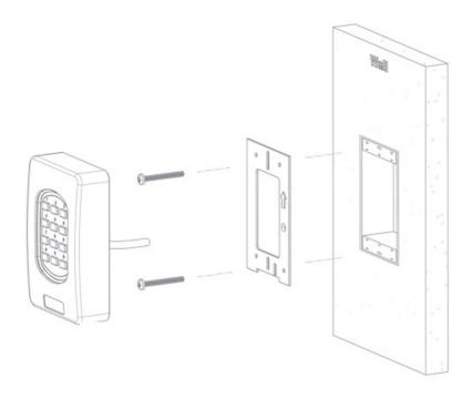
For a wall mounted installation, locate the electrical box which will be recessed into the wall. You will see a top and bottom metal flange with holes which is used to secure the back plate to the wall. Using the Phillips machine screws provided (#6- 32 x .375") screw the back plate against electrical box so that it's flush.
