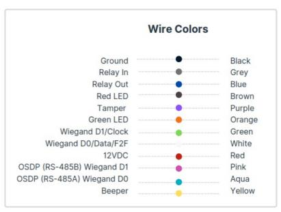
The next step is to connect the wires as per the wiring table above.
