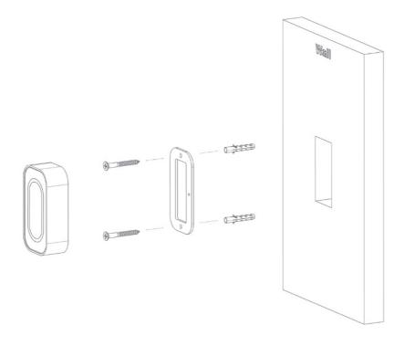
For a wall-mounted installation, beginby pre-drilling your holes and inserting the nylon screw plugs provided to support the weight of the reader. Once secured to the wall, you can fix the black plate to the wall using the screws (SCR PTP, 2X6MM BLUE, ZINC CR3) provided.
