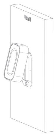
Once the back plate has been fitted and the wiring is complete, the top casing can be inserted onto the bottom casing as shown above.
