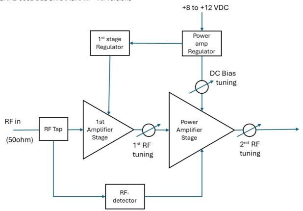
The SAFE-0002 is a 2 stage fixed gain amplifier. A linear regulator supplies the power to the first stage preamplifier and the second stage is supplied with the external power input – typically +8 to +12 VDC. The circuit is designed to provide gain of approximately 20 to 30 dB. This common circuit can be tuned to operate in the range from 150 MHz to 940 MHz. The tuning is performed in the factory prior to shipping. The user can not change the tuning.
