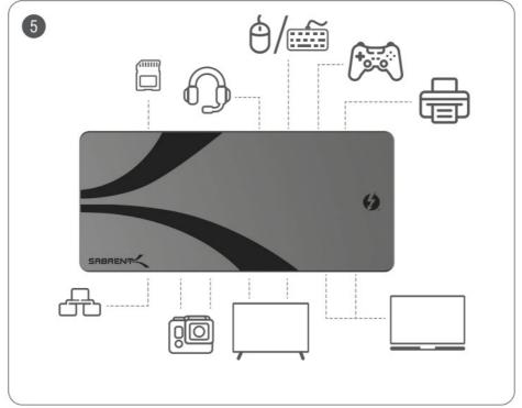
Insert any microSD and/or SD memory cards into the memory card slot(s) and connect any USB peripherals for use or for charging.
