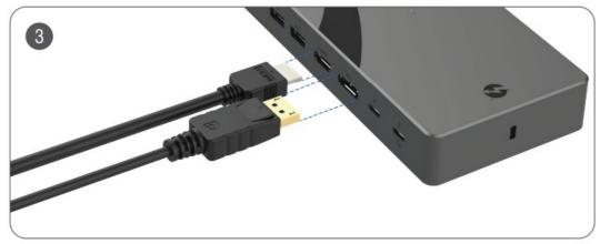
Connect external displays through the HDMI, DisplayPort (DP), and/or Thunderbolt 4 (TB) ports.
