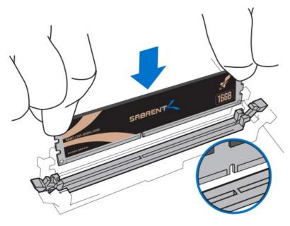
Using firm, even pressure, push DIMM into slot until clips snap into place. Do not assist clips.
