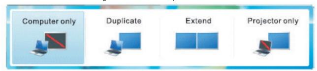
**Note:** Windows 7 has a projection menu feature that enables you to quickly connect your laptop to a projector or an extended monitor
