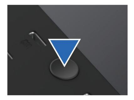
To turn the screen on or off, press and hold the function button for 2 seconds.
