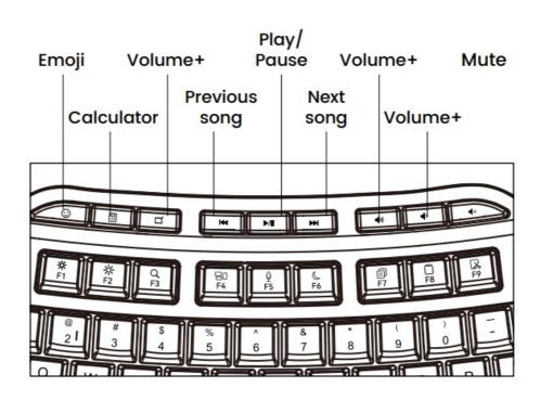
A single function key that triggers the function directly when pressed.
