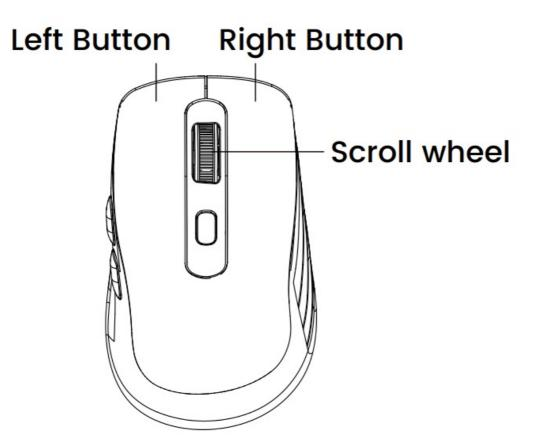
Press and hold the left, middle, and right buttons of the mouse until the indicator light flashes, then plug the USB into the computer.
