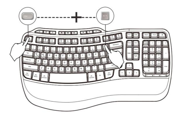
**Pairing method:** Long-press the "ESC" + "=" keys for three seconds until the red light flashes. Then, immediately plug in the receiver.
