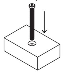
• **D**: Align the Bolt and Feet assembly with the threaded holes on the underside of the Seat Platform.
