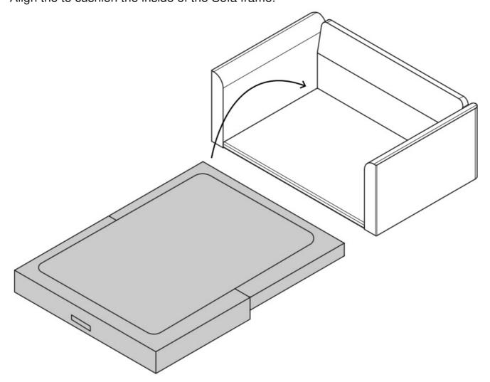
• **B**: Fold the Cushion, pulling the back edge of the cushion to the inside of the Sofa and pushing down.
