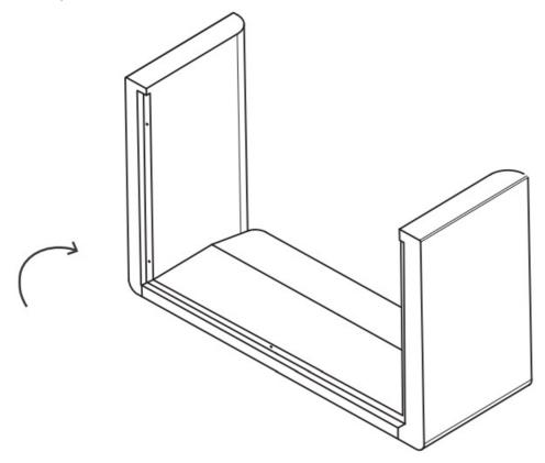
• B: Align the Seat Platform to the bottom of the Back and Arms. There will be a cut out
