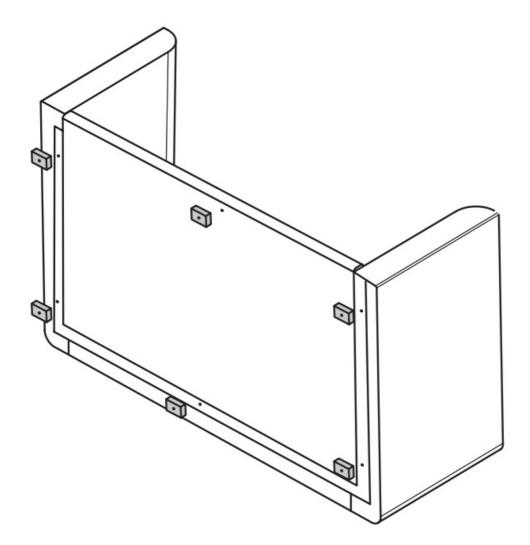
• E: Using the Ratchet Wrench, loosely tighten each bolt first before tightening all the way.
