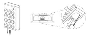
2. Load 4 AAA batteries correctly, squeeze the clamp and push the battery holder into the compartment, then tighten it with the screw.
