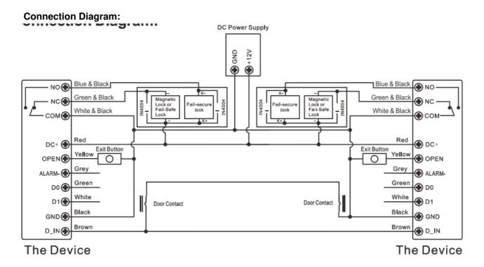
**Remarks**: The Door Contact must be installed and connected as the diagram. Let's name the two Devices as "A "and "B" for two doors "1" and "2"
