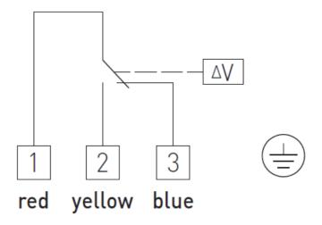
flow > switch-on value no flow existing (flow falling below the preset switch-off value)
