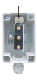
Mechanical wind vane switch RHEASREG® WFS with switching output, in an impact-resistant plastic housing, with stainless-steel paddle, for flow monitoring of gaseous, non-aggressive media. The flow sensor is used as a flow controller or air flow monitor in air conditioning ducts, in air intake or exhaust devices of ventilators or electric heating registers (also for contaminated, oily air).
