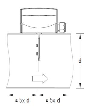
The installation is only possible in horizontal air ducts!
