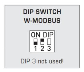
The connection type is set via pos. 1 of the "W-Modbus" DIP switch – see table! The operating mode is set via pos. 2 of the "W-Modbus" DIP switch – see table! To use it as a master gateway (base station on DDC/PLC), DIP 2 must be set to ON. If the unit is switched over, it is unpaired and must be paired again in the network. Pos. 3 of the "W-Modbus" DIP switch is not used.
