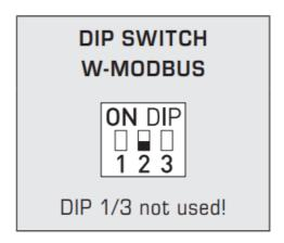
The operating mode is set via pos. 2 of the "W-Modbus" DIP switch – see table!
