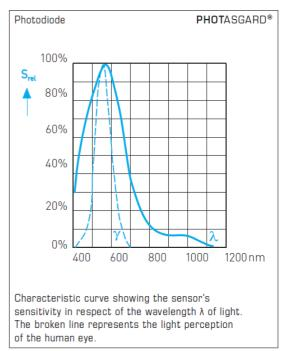
The sensor used in PHOTASGARD® light intensity sensors (photodiode) was specifically adapted to the sensitivity of the human eye. Its greatest sensitivity is in the range of 350 nm to 820 nm. Therefore with its special filter the sensor is predestined for exposure measurement of daylight and / or for measuring artificial light of high color temperature (similar to sunlight).
