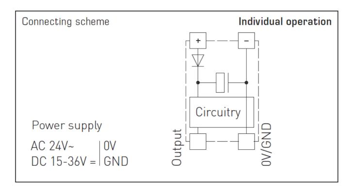
When several devices are supplied by one 24 V AC voltage supply, it is to be ensured that all "positive" operating voltage input terminals (+) of the field devices are connected with each other and all "negative" operating voltage input terminals (–) (= reference potential) are connected together (in-phase connection of field devices). All outputs of field devices must be referenced to the same potential!
