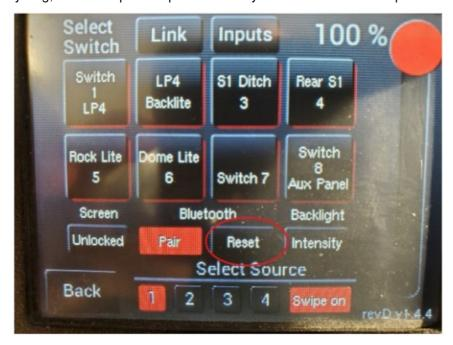
• **Touchscreen:** Press the "Setup" button on the home screen, then press and hold the "Reset" button in the Bluetooth menu for 5 -6 seconds until the "Pair" button illuminates red, this will clear any previous device pairings, and put the touchscreen in pairing mode for 60 seconds.
