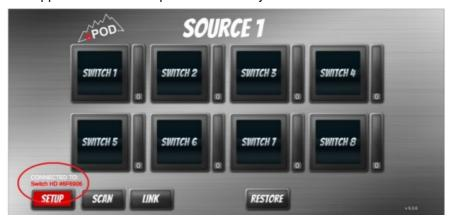
• Once connected, app will show "connected to Switch HD" in the bottom left corner of the screen
