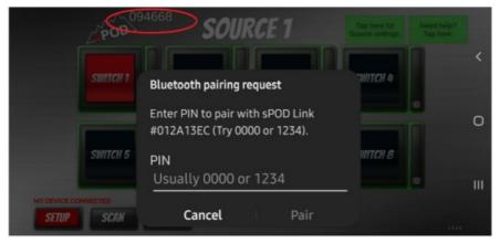
• The app will Pop up a PIN entry screen, press "Cancel", then "Setup" and "Scan" again. After approx. 6 seconds, a 6-digit PIN number will appear on the top left center of the screen next to the S-Pod logo, and the PIN entry screen should appear again (On Android devices, you may need to perform this part of the procedure 2-3 times to get the PIN number to display).
