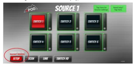
• Enter the PIN number and select "Pair" the app will say "pairing" and connect to the selected device and populate the "connected to" location on the bottom left corner of the screen.
