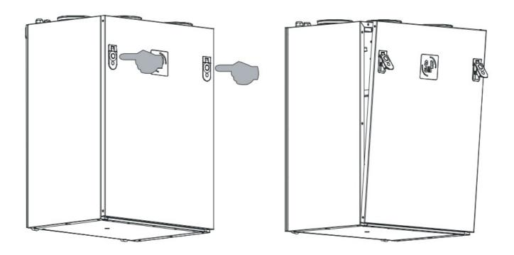
For security reasons the unit has an integrated electro magnetic door switch which disconnects the power supply when the door is opened.
