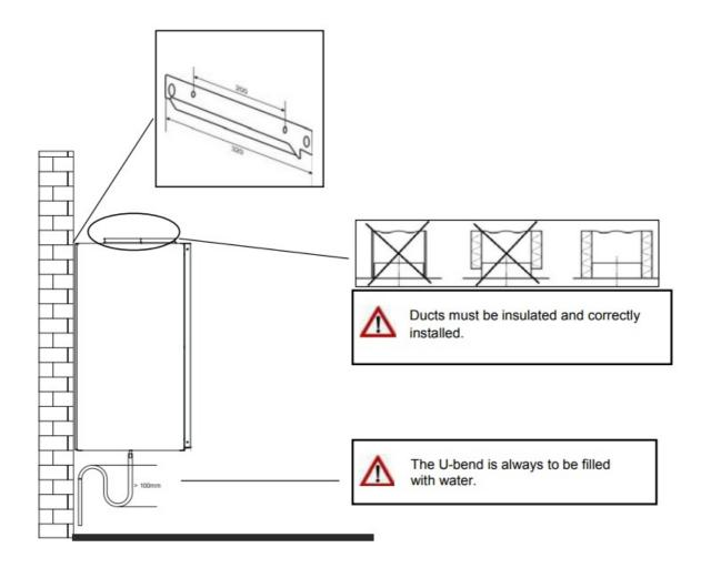
The CAD HE 325/450/575 heat recovery unit is designed for indoor installation.
