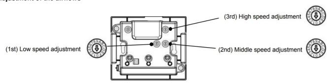
To adjust the airflow turn the potentiometer carefully clock wise with a small screw driver. The potentiometer has 16 positions (from 0 to F). To each of these positions are assigned an output voltage to the fans. As higher the output voltage as higher the airflow and vice versa.
