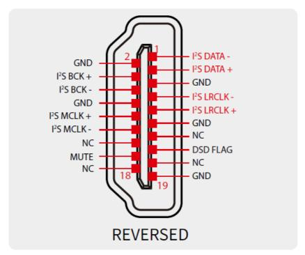
• REVERSED (INVERTED, DATA AND LRCK INVERTED)
