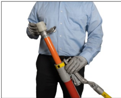
Figure 20. Resetting the Loadbuster tool.
