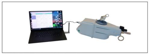
Figure 10. Completed TripSaver II recloser setup.
