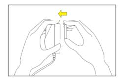
Figure 8. Install the plug adapter.
