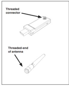
Figure 4. Connecting the antenna to the USB transceiver.
