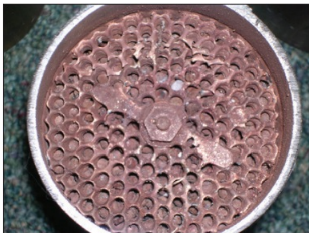
Figure 6. Silencer after three operations at full fault current.
