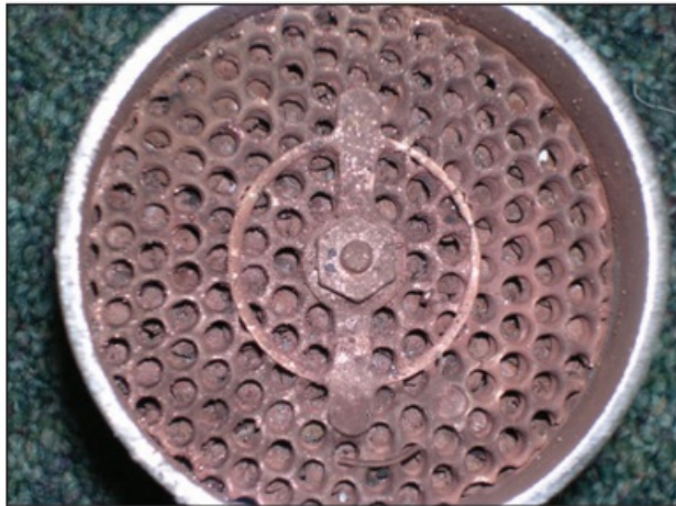
Figure 5. Silencer after one operation at full fault current.
