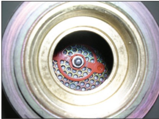
Figure 4. Silencer with a red wear indicator.
