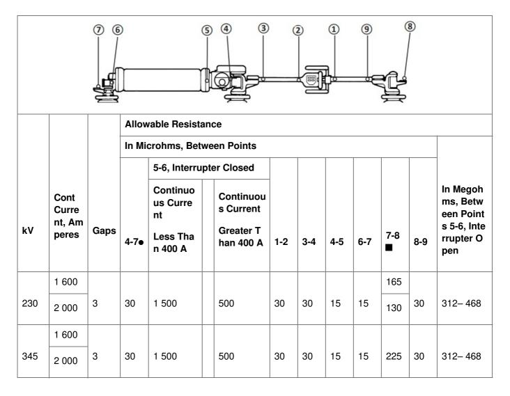
The resistance between points 4 and 7 minus the actual measured resistance between points 5 and 6 with the interrupter closed.
