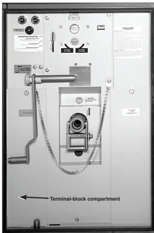
Figure 9. Left side of low-voltage control compartment showing location of left terminal-block compartment—right terminal-block compartment similar—for connection of leads from S&C Current Sensors furnished with optional overcurrent lockout and for customer connections when optional auxiliary switches, remote indication, or supervisory control is furnished. Terminal blocks for options “-Y4” and “-Y6” are in the left terminal-block compartment only.
