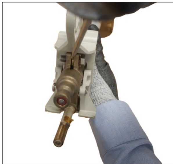
Figure 5. An SMD-20 Power Fuse upper ferrule without a bronze spacing washer.
