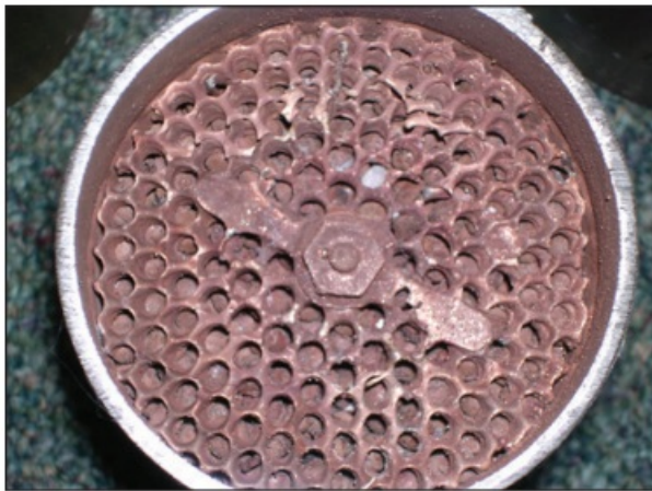
Figure 9. Silencer after three operations at full fault current.
