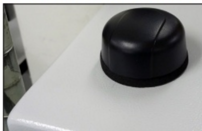
Figure 7. Exterior view of the installed GPS antenna.
