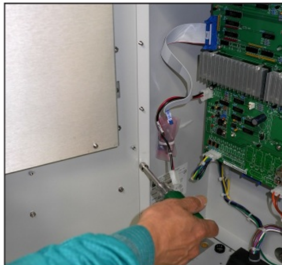
Figure 4. Remove the front panel attachment nuts.
