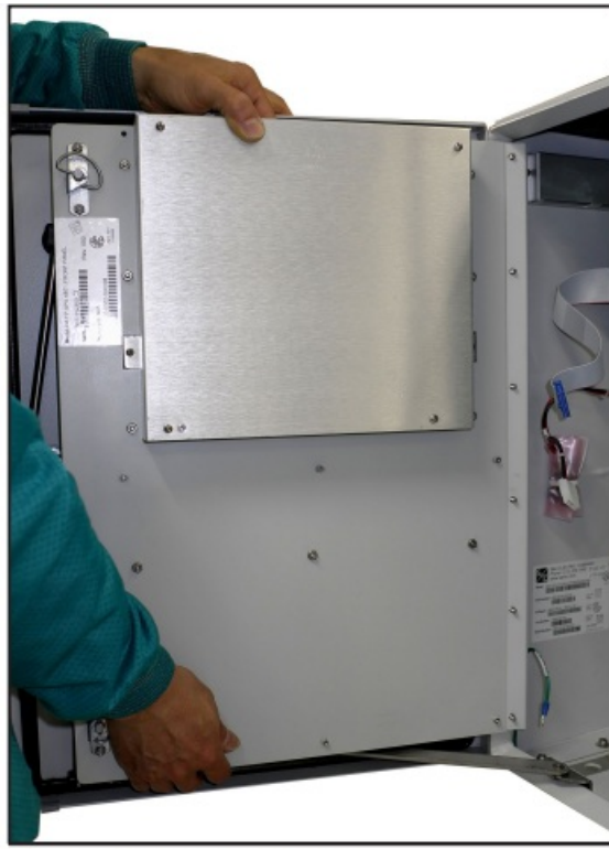
Figure 5. Remove existing front panel.
