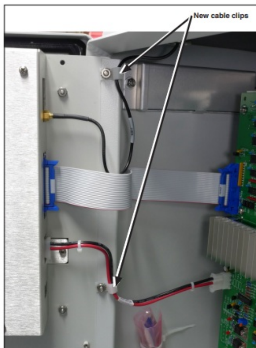
Figure 9. Locations of the new cable clips.
