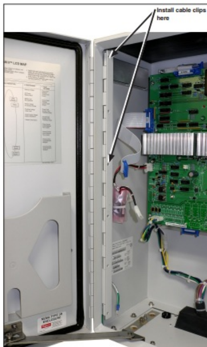
Figure 8. Cable clip locations at the front panel.
