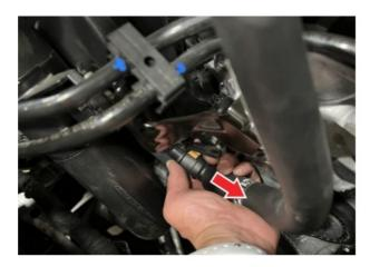
Loosen the hose clamp connecting the intake tube to the turbo inlet. Tools Required: 7mm Deep Socket with 3" Extension
