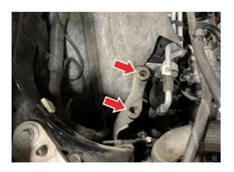
Using adjustable pliers, expand the bypass hose clamp by squeezing the tabs together and remove the hose from the bypass valve. Set the hose clamp aside to be reused later.
