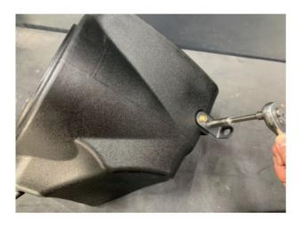
Remove the shoulder bushing and grommet from the stock intake box and install them to the Box Bracket (2). Note the orientation of the grommet and bushing when installing them to the Box Bracket.
