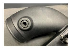
Remove the IAT sensor from the stock intake. Lean the IAT Sensor back as you rotate it counterclockwise so that the tab on the sensor goes over the locking ramp. Once the sensor tab is passed the locking ramp it can be pulled out and removed.
