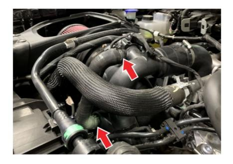
Install the connector onto the IAT sensor. If your connector harness is not long enough to easily connect to the sensor, use the provided Harness Extension (20) and use Cable Ties (21) to hold the extra length together so that it is secured away from any hot or moving components and also not rubbing against any components.
