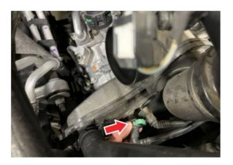
Remove the smaller vapor quick connect fitting from the intake tube. Depress both green tabs to release and remove the quick connect fitting.
