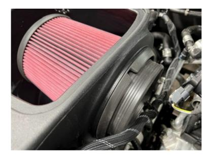
Place the Gasket (14) on to the Tube (11) making sure the holes line up with the threaded holes in the Tube.
