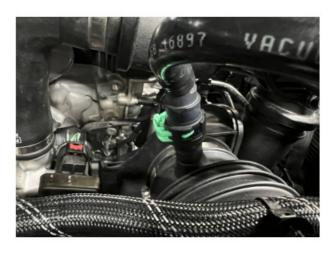
STEP 6 Loosen the hose clamp attached to the flexible coupler.
