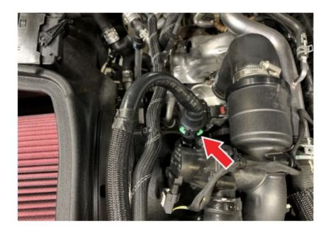
Install the dual quick connect hoses. Make sure the green locking tab is engaged in the larger quick connect after installing the quick connect hose. Make sure the smaller quick connect locks into place as well.
