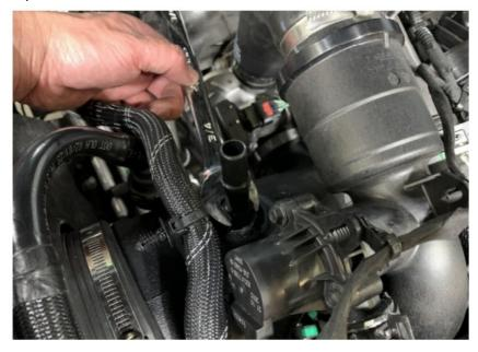
Install the Wrapped Hose (17). The Wrapped Hose will have a sharper 90 degree bend and a lesser 100 degree bend. The end with the sharper 90 degree bend will be installed on the Tube (11) and the lesser 100 degree bend will install onto the bypass valve. Place the factory hose clamps over the Wrapped Hose in a position so you can install both ends of the Hose.
