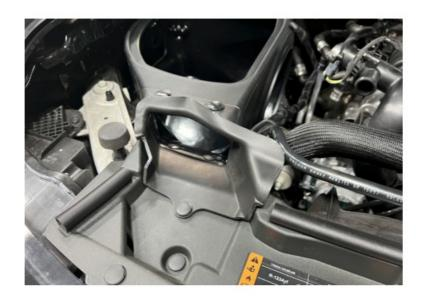
Install the Filter (7) into the Intake Box (1). Insert the Filter flange first through the top opening of the Box. Center the Filter flange with the round filter opening of the Box. Make sure that all around the tip of the tapered snap-in feature of the filter is inside the round filter opening before you use the filter flange to pull the filter until the tapered feature completely snaps around the outside of the round opening.
