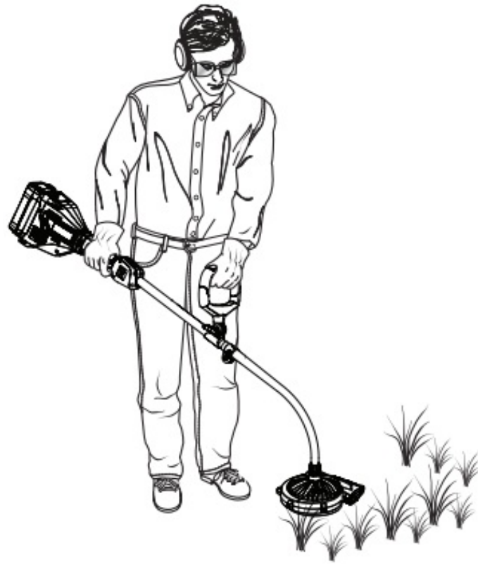
Fig. 9 PROPER STRAIGHT SHAFT TRIMMER ATTACHMENT OPERATING POSITION
