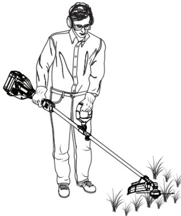
Fig. 9 PROPER STRAIGHT SHAFT TRIMMER ATTACHMENT OPERATING POSITION
