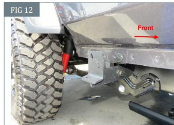
(Fig 12) Attach the Passenger/Right Rear Bracket and Passenger/Right Rear Support Bracket to the rear location
