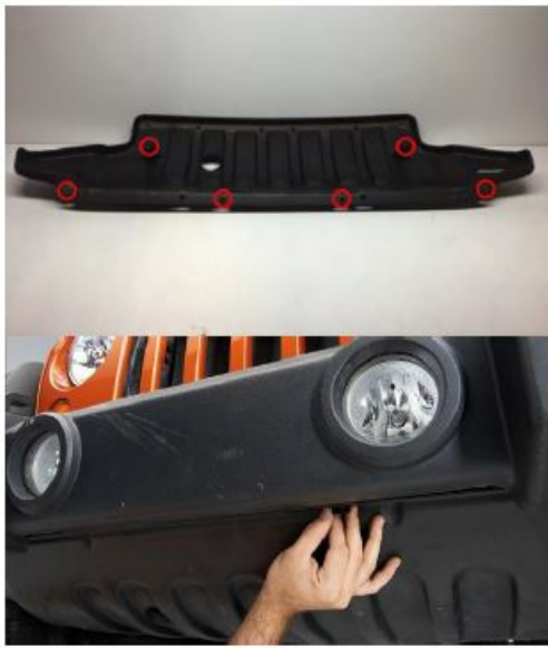
(Fig 1) Remove the (6) plastic push pins securing the factory splash shield to the vehicle
