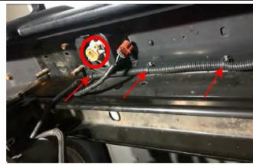
(Fig 2) From under the vehicle, remove the factory fog light connectors and free the fog light wiring loom from the bumper.
