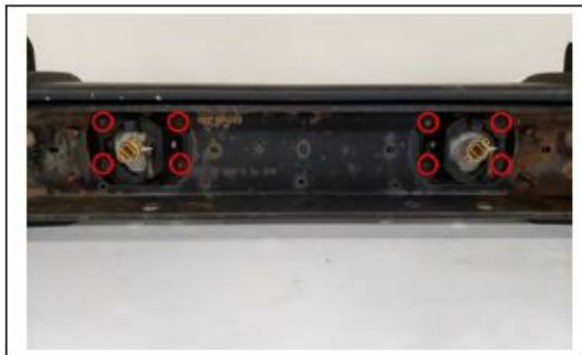
(Fig 5) Remove the (8) 7mm screws securing the fog lights to the factory front bumper.
