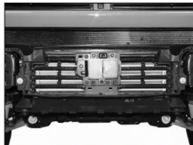
(Fig 6) Remove the shutter assembly. Models with ACC sensor (pictured), unplug and remove sensor from shutter assembly
