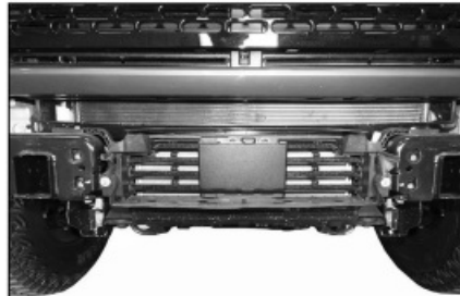
(Fig 4) Remove factory hex bolts from front to remove bumper assembly
