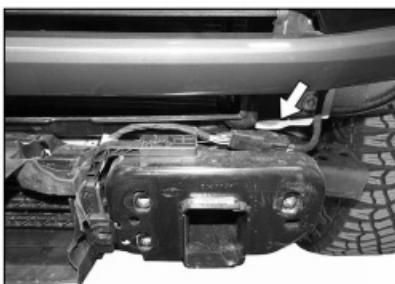
(Fig 5) Unplug harness leading to shutter assembly (arrow)
