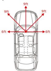
Scenario 2: Install the proximity sensor on the front windshield vertically, facing rear.
