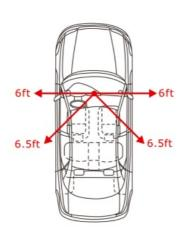
Scenario 3: Install the proximity sensor on the roof of car in horizontally, facing down.
