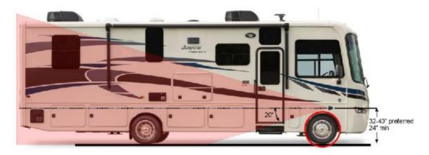
With the wheel well, be sure that the viewing angle does not overlap it in any way. You may adjust the height or move the sensor slightly back if needed. It is recommended to have the sensor as forward as possible while avoiding the wheel well and staying near the preferred height.
