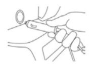
5. [Audio Prompt: Push the Auto Position button] The Auto Position process automatically positions RVibrake3 in the seat pan of the towed vehicle, and removes vacuum stored in the towed vehicles braking reservoir.
