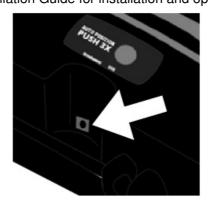
**IMPORTANT:** Any time the towed vehicle's engine is started after setup of RVibrake3, the Auto Position process must be completed again to drain the vacuum in the braking reservoir.
